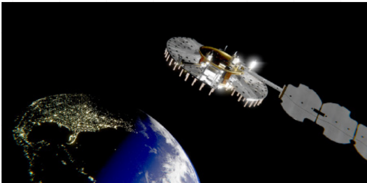
Artist's concept for NTS-3 in geostationary orbit. L3Harris Corporation will integrate NTS-3 using Northrop Grumman's ESPAStar bus, building on EAGLE's flight heritage. Graphic Credit: 1st Lt. Jacob Lutz
