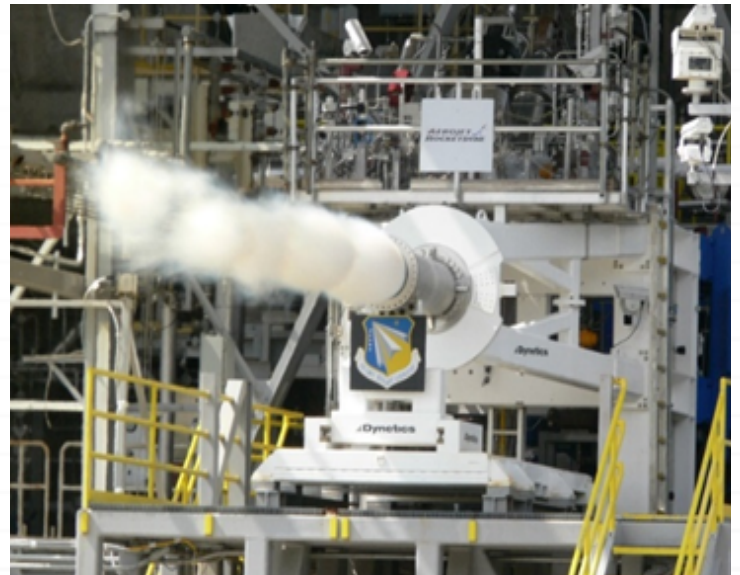
HydroCarbon Boost Preburner test. NASA Stennis Space Center (2019)
