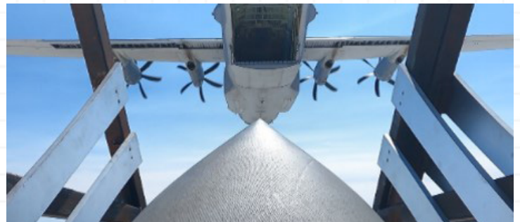
An airdropped Palletized Munition Deployment System. The photo shows one of the cruise missile simulants in the Deployment Box immediately after being airdropped from a MC-130J. (Courtesy photo)
