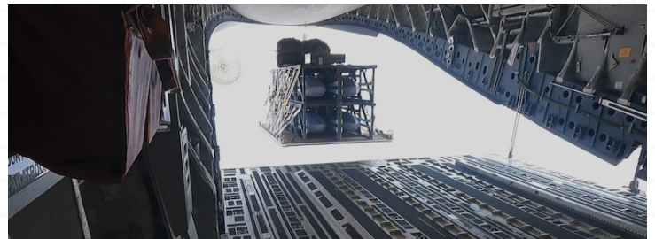
A standard cargo airdrop of the Palletized Munition Deployment System from a C-17A. A four-pack configuration is used for demonstration purposes. (Courtesy photo)
