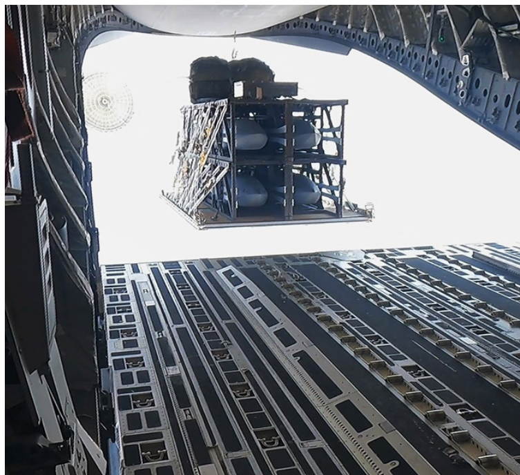
A standard cargo airdrop of the Palletized Effects Deployment System from a C-17A. A 4-pack configuration is used for demonstration purposes. (Courtesy photo)
