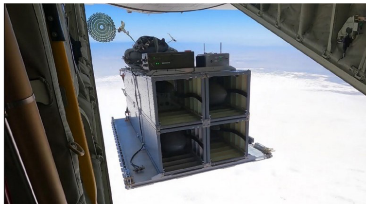
Rapid Dragon Operational Prototype, which was integrated on a USMC KC-130; this was the first time Rapid Dragon was integrated and demonstrated outside the USAF. The photo shows a heterogeneous loadout flight test conducted in a SDPE / USMC partnership. Photo is from a flight demonstration (April 2023). (Courtesy photos)
