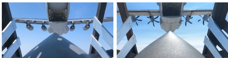
Palletized Effects airdrop. The photos show a cruise missile simulant in the Deployment Box immediately after being airdropped from a C-17A (left) and an MC-130 (right). (Courtesy photo)
