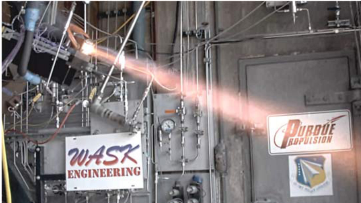
ARMR risk reduction: Methane Aerospike Thruster testing at Purdue, Nov 2019.
