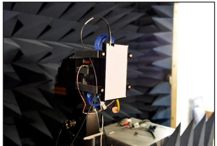
A custom-built AESA mounted to an antenna positioning system during beam pattern characterization measurements. Photo Credit: AFRL
