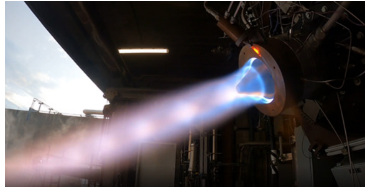
22,000 newton thrust (5000 lbf) RDRE testing with liquid oxygen and gaseous methane testing by AFRL partner IN Space LLC at Purdue University in 2021.
