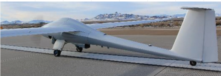
Picture of ULTRA on runway preparing for takeoff. Current upgrades will push the endurance to potentially greater than 80hrs depending on payload.
