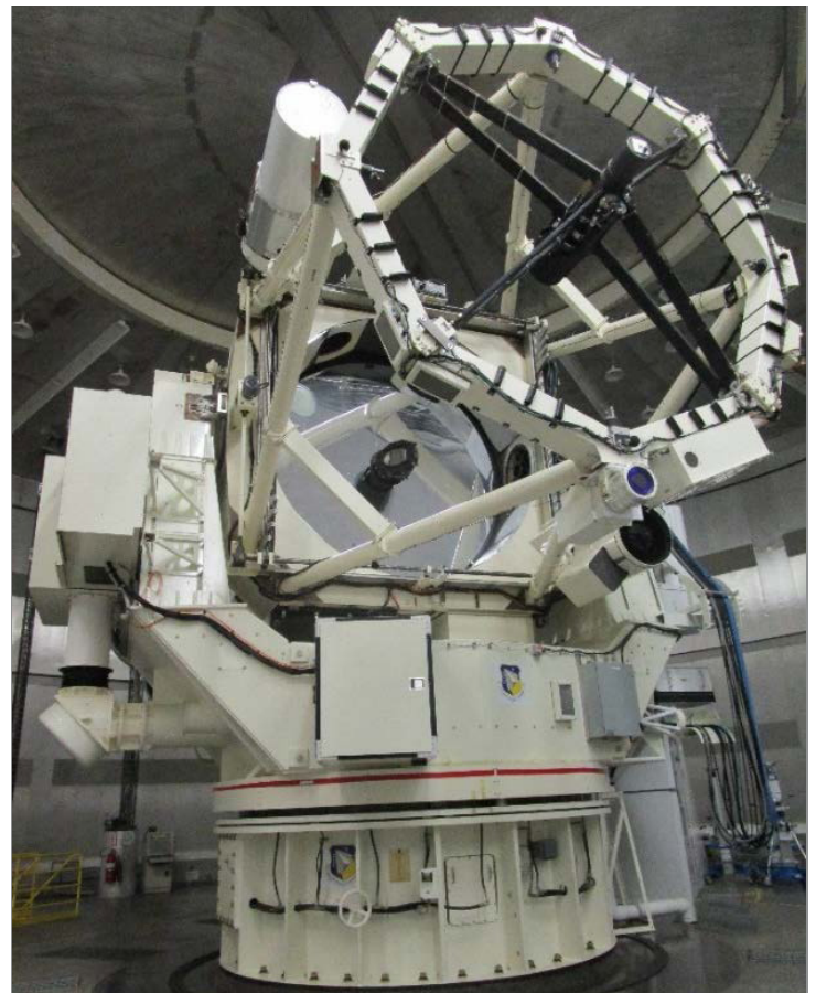
The 3.6-meter, 75-ton Advanced Electro-Optical System (AEOS) telescope shown above is the largest optical telescope in the Department of Defense. In addition the Maui Space Surveillance System facility houses several other telescopes ranging from 0.4 to 1.6-meters. Photo credit: AFRL
