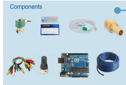
Ventilator components include (left to right, top to bottom): 12 VDC brass solenoid valves, breadboard/wire kit, oxygen reservoir, barbed hose fitting, alligator clip leads, air regulator, Arduino Uno microcontroller board, air hose
