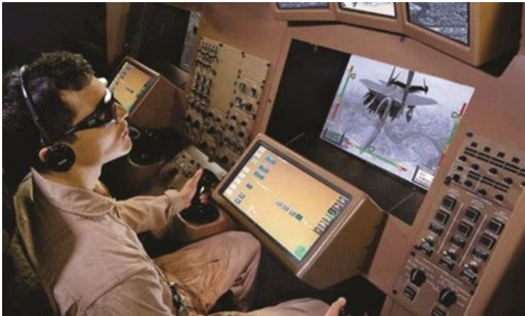
KC-46 Air Refueling Operator Station showing RVS 1.0 design with HD resolution, black and white cameras and 3D display.
