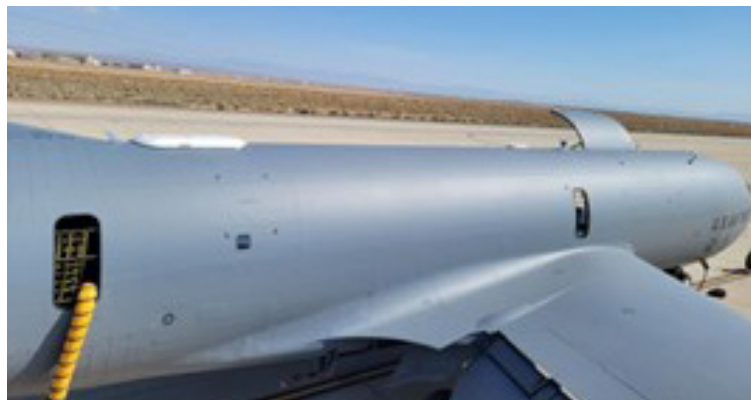
A KC-135 preparing for flight test of a pLEO SATCOM system. Note the low-profile phased array antenna.
